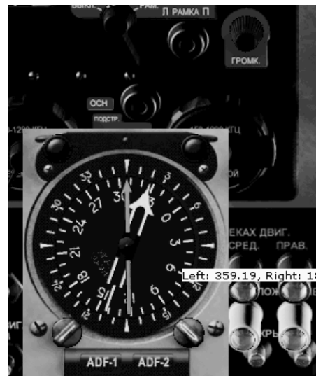
3. Begin to measure the bearing of ADF-2 active freq.
