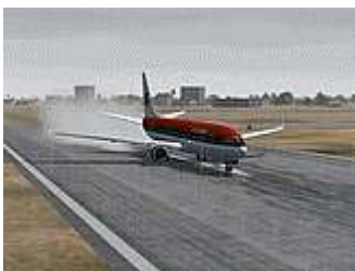
If the runway is wet and thrust is at 35% or above, water will spray up behind the engines
